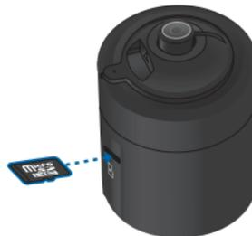
To remove the microSD card, push the card in to release the lock. Pull the card out.
