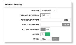
**Auth Server IP/Port** In the first field, enter the IP address of the RADIUS authentication server. RADIUS is a networking protocol providing centralized Authentication, Authorization, and Accounting (AAA) management for computers to connect to and use a network service.
