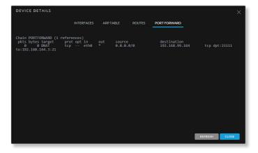
Port forwarding allows you to connect to a specific service such as an FTP server or web server. Port forwarding creates a transparent tunnel through a firewall/NAT, granting access from the WAN side to the specific network service running on the LAN side.
