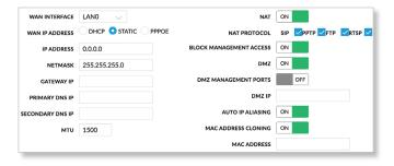
**IP Address** Enter the IP address of the device. This IP will be used for device management purposes.
