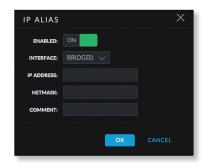
Enabled Select this option to enable the specific IP alias. All the added IP aliases are saved in the system configuration file; however, only the enabled IP aliases are active on the device.
