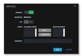
Enabled Select this option to enable the specific bridge network. All the added bridge networks are saved in the system configuration file; however, only the enabled bridge networks are active on the device.
