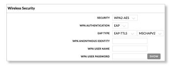
**EAP Type** Select the authentication protocol (**EAP-TTLS** or **EAP-PEAP**) and the inner authentication protocol (**MSCHAPV2**).
