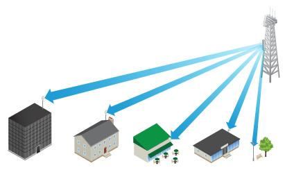
The PowerBeam used as a CPE device for each client in an airMAX PtMP network.
