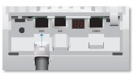
2. Create a strain relief for the Ethernet cable by feeding a cable tie through the tie slot under the cable. Then wrap the cable tie around the cable and tighten.
