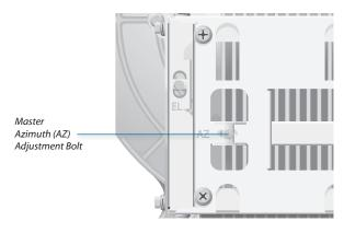
b. Sweep the *Elevation (EL) Adjustment Bolt* of the *Master* through its adjustment range.
