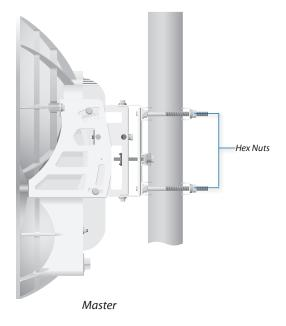
4. Slave Aim the *Slave* at the *Master* to achieve the strongest *Signal Strengths* for the *Slave*. If necessary, adjust the *Slave*'s position on the pole.
