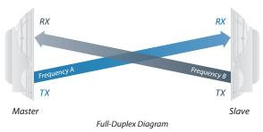
• **TX and RX Frequencies** The *TX Frequency* on the Master must match the RX *Frequency* on the Slave, and vice versa.
