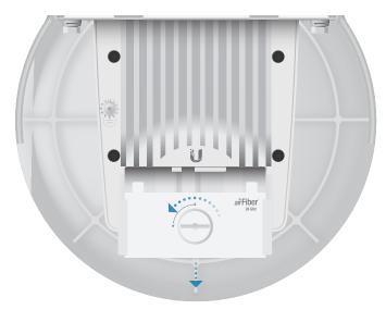
5. Connect the External GPS Antenna to the GPS SMA connector.
