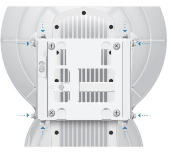
4. Ensure that there is a 6 mm (0.24 in) gap between the head of each *Serrated Flange Screw* and the *Alignment Bracket*.
