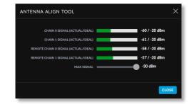
Note: The *Signal Strength* bar graphs display the absolute power level (in dBm) of the received signal for each chain. Lower values indicate stronger received signal levels.
