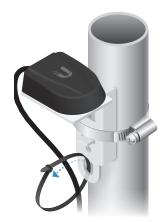
4. Turn the Cover Lock counterclockwise to the Unlocked ■ icon. Slide the Port Cover down to remove it.
