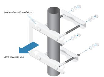
3. Loosen, but do NOT remove the eight *Lock Bolts* located on the *Alignment Bracket*.
