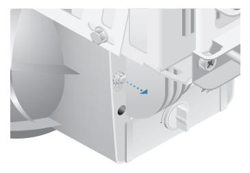
2. Attach a ground wire (min. 8 AWG or 10 mm<sup>2</sup>) to the lug and replace the nut to secure the wire.
