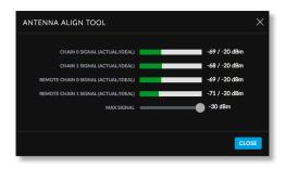
Use the *Align Antenna* tool to point and optimize the antenna in the direction of maximum link signal. (See **"Using the airFiber Configuration Interface" on page 15** for more details.) The *Antenna Alignment* window reloads every 250 milliseconds.
