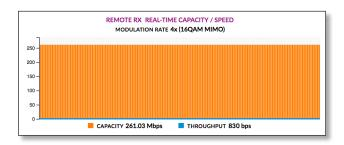
The capacity is the expected maximum rate at which data can be transmitted over the channel (accounting for protocol overhead and interference).
