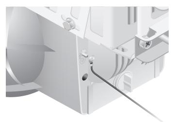
3. Secure the other end of the ground wire to a grounded mast, pole, tower, or grounding bar.
